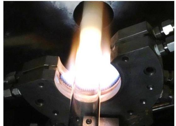
strength due to moderate flame pressure. It does not require any setting of individual tips, characteristic for multi-tip type of burners. Matrix for gas delivery and mixing is available as spare part and can be exchanged easily. High outer edge may require installation at a small inclination angle in the horizontal plane, to provide proper visibility of the
