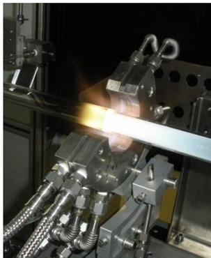
**CVD-08 preform glass working lathe is used for:** preparation of substrate tubes, fire polishing of preforms before fiber drawing, preform jacketing, stretching and reforming, collapsing and consolidating PM fiber preforms and consolidation of microstructured preforms.
